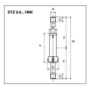
These special KD and STZ transducers are used to check out material testing machines and are designed in accordance to ISO 376. They are compressive force transducers and tensile force transducers that, because of their maximum overall height, are suitable for checking material testing machines according to ISO 7500-1.
